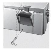
Opening for adjusting the column guide, with 6 mm internal socket spanner.
