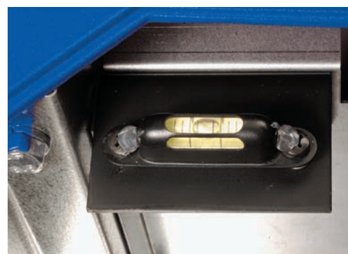
3. Spirit level for accurate testing on uneven floors (DLX version).
