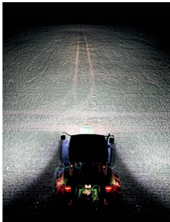
Upgrade Option 3: The Future 6 x LED work lamps Alternator load 11.0A
