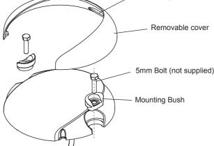
If passing the cable through a hole, ensure there are no sharp edges to cut or chafe the cable.
