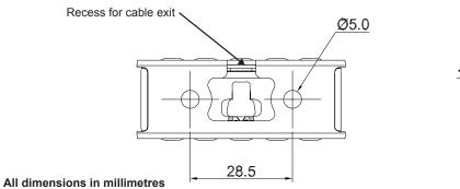
Note: Mounting bolts need to have a head height less than 3mm.
