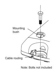
Note: When mounting lamp units side by side allow a gap of 5mm to ensure screw cap removal.
