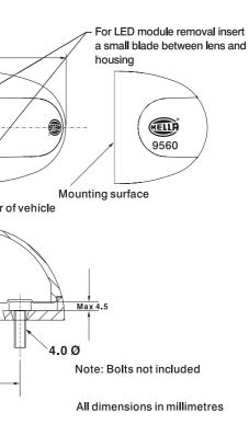
The LED module is securely fastened to prevent dislodging in service, and removal would not normally be required. If it becomes necessary to remove the module, insert a small blade on both sides of the LED module and the housing at the correct position and prise the module free from the housing (See diagram above).
