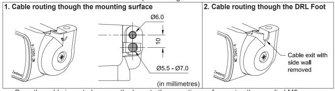
Once the cable is routed, secure the lamp to the mounting surface using the supplied M5 screws, washers and nuts.
