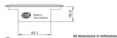
Note: Lamp may be mounted in the horizontal or vertical postion.
