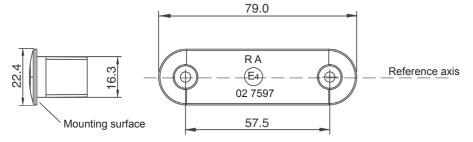
Note: Lamp may be mounted in the horizontal or vertical postion.
