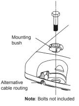
**Note:** When mounting lamp units side by side allow a gap of 5mm to ensure screw cap removal.
