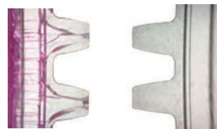
Stress cracked PC.
