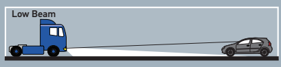
Low Beam Designed to light the road at night without causing glare to other road users.
