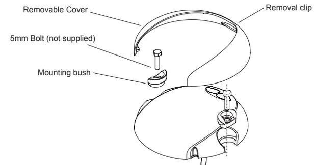
Clip the cover on securely until flush with the lamp surface.
