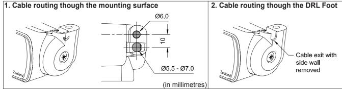
Once the cable is routed, secure the lamp to the mounting surface using the supplied M5 screws, washers and nuts.
