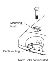
Note: When mounting lamp units side by side allow a gap of 5mm to ensure screw cap removal.
