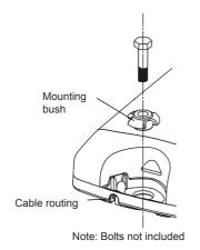
Note: When mounting lamp units side by side allow a gap of 5mm to ensure screw cap removal.
